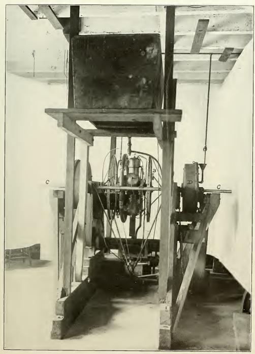
DYNAMOMETER TESTS OF LARGE ENGINE
